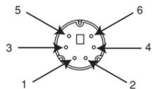
\*Above figure shows the pin assignment seeing the Clamp sensor from output connector part. The figure of the pin assignment of connection terminal is symmetrical to above figure.
