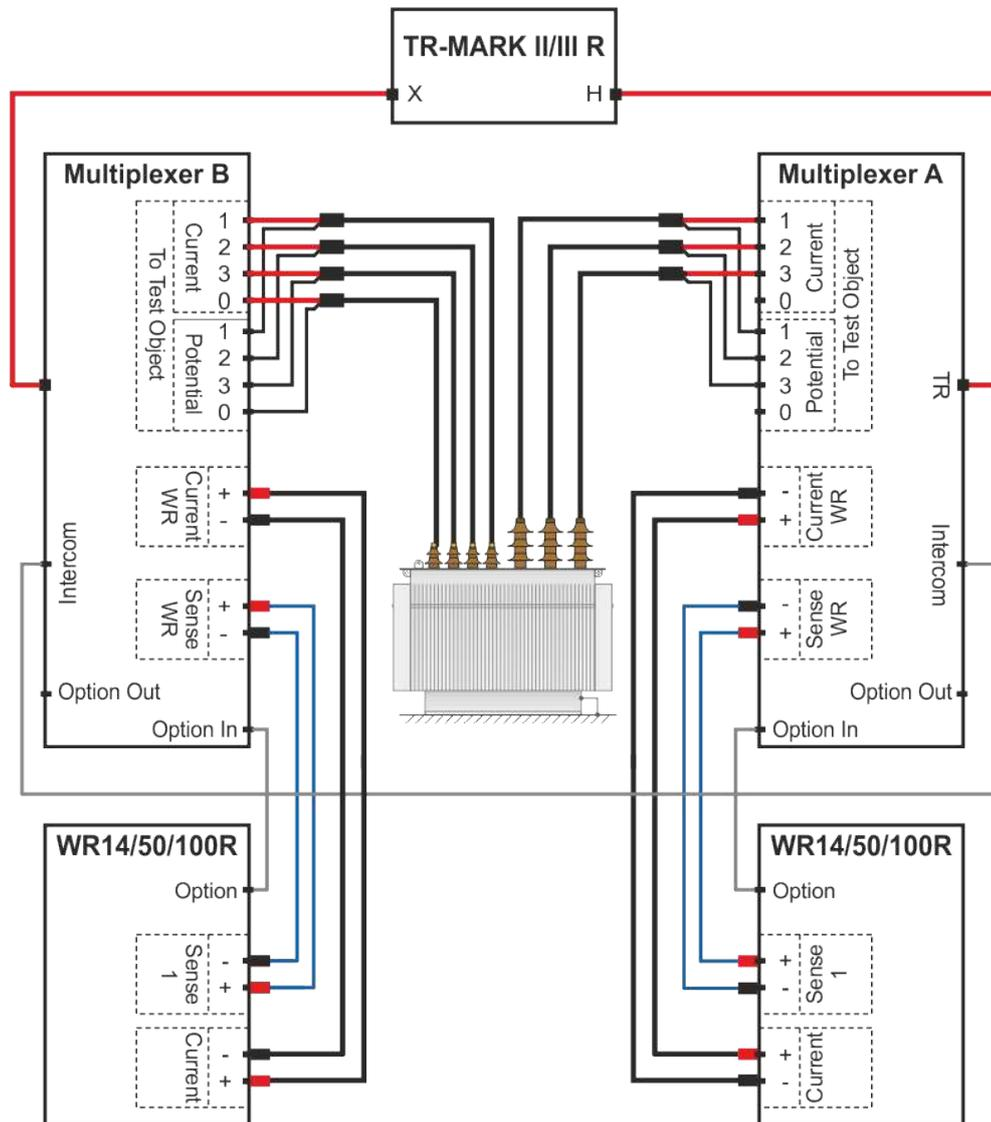
Often primary and secondary winding systems have very different winding resistances. To get reliable results, different currents ranges are needed for the two winding systems. If you add a second WR to the example in chapter '4.2' you get the possibility to measure both winding systems with different currents at the same time.
