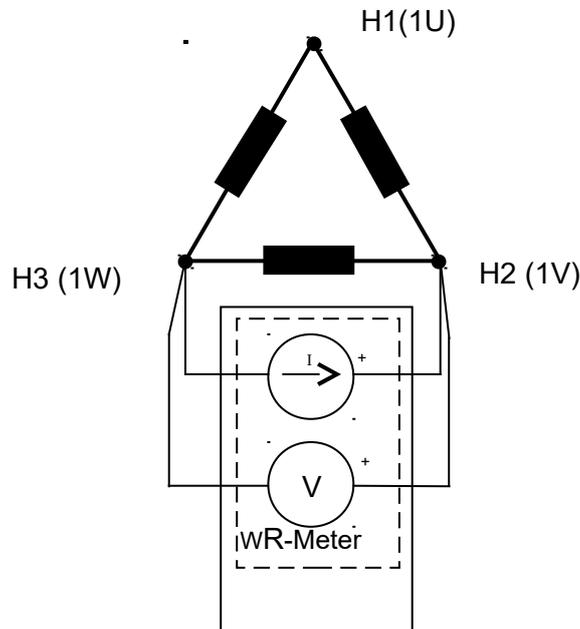
Current Terminals are represented by a current source and Sense terminals are represented by a Voltmeter.
