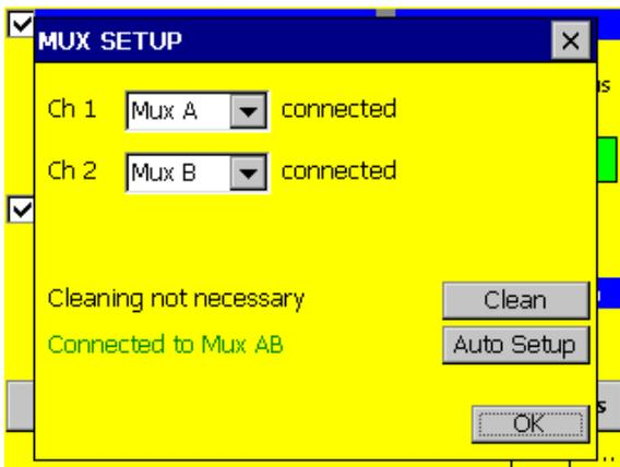
Every available Channel on the controlling Winding Resistance Meter will be displayed, with a combobox where you can select your options
