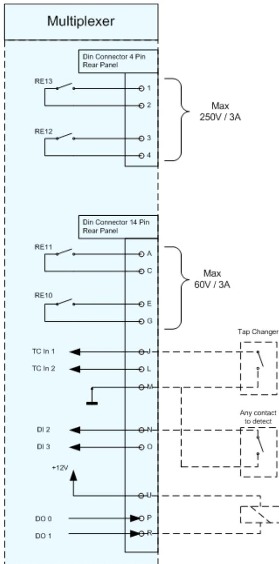
Every Element in the ,Multiplexer' field can be set or read by the controlling WR unit or its remote control.
