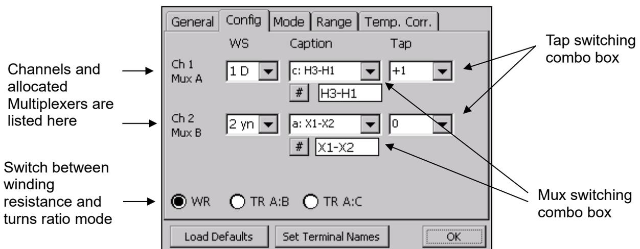
Because of the transformer profile, a Raytech winding resistance meter knows how to switch a Multiplexer to measure a transformer. By touching the Mux switching combo box, a selection of possible relay configuration appears.
