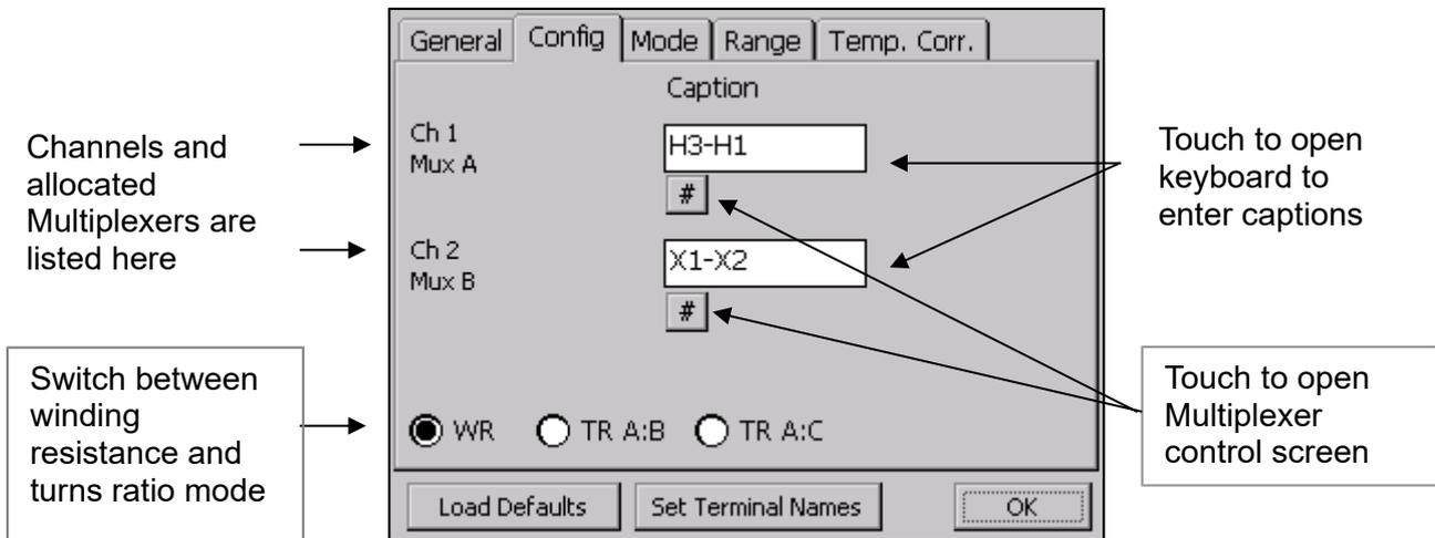
When the **#** button is touched as described above, a simple screen to control Multiplexer with a dot matrix is opened. This is the way, to switch a winding resistance meter to any test object. It's recommended when the device under test is no transformer. The following page shows how this screen looks, and how explains how to use it.
