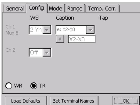
Switch Mux B and C to TR
