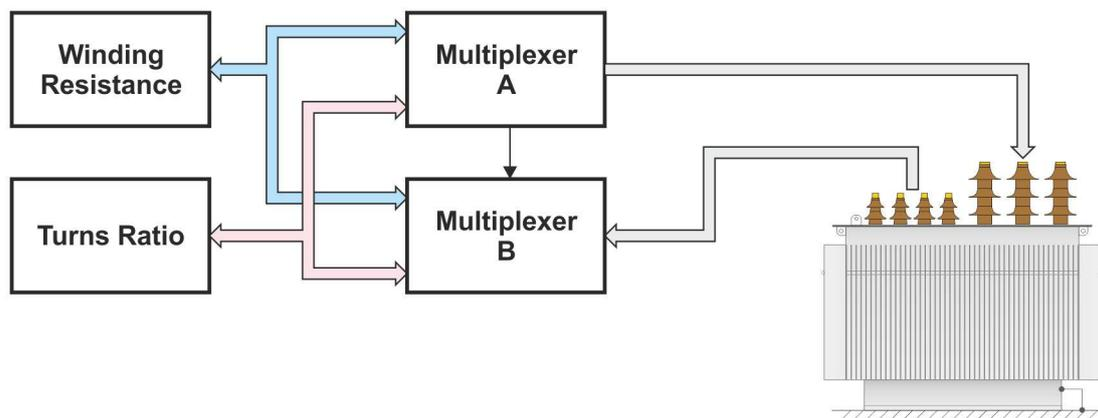
Multiplexers are directly connected to the test object. Raytech Meters are connected to Multiplexers. It is the interface between transformer and instruments.
