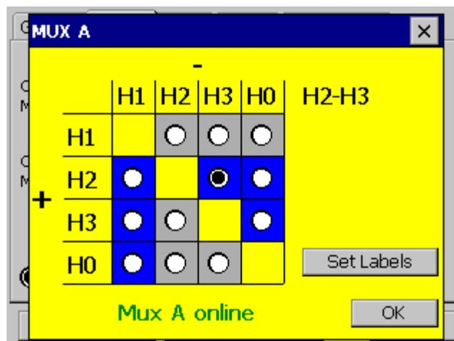
The displayed matrix shows, how your Winding Resistance Meter is switched to the connected transformer or other test object. Current and potential (channel) are always switched to the same configuration.
