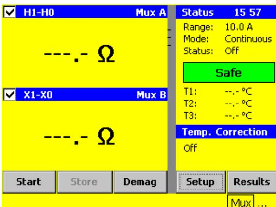
When a multiplexer is connected successfully to a Winding Resistance Meter, and it is allocated in the actual Multiplexer configuration, an indication 'Mux' plus the address letter A to C will be displayed in the affecting channel header. This 'Mux' text works also as a direct link button to the multiplexer control screen.
