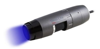
The AM4115-FUT, with the exceptional image quality of Dino-Lite Edge featuring 375nm UV lighting with high sensitivity 1.3 Megapixels sensor., is designed to meet more professional needs. It also has better adaptability to different applications with the detachable and exchangeable front cap design.
