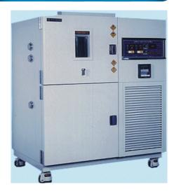
It is a device for testing the reliability of various parts and products, It tests thermal characteristics of a component and product by rapid temperature change.
