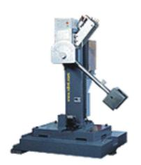
Test equipment to measure energy absorption
