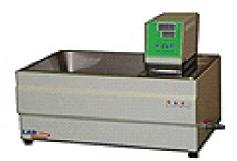
It is a tester for the quality and physical properties of various materials at a high temperature in water, and it is possible to control the temperature accurately by Digital P.I.D Controller system.
