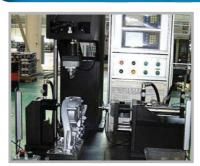
This equipment is used to simultaneously produce and inspect PIN with AL die casting products at a constant load / depth.
