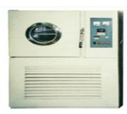
This device inspects the crack the sample in an experiment at low temperature. Through the sight window the inside can be observed.
