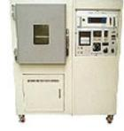
It has been designed / manufactured for the purpose of measuring heat deterioration of vulcanized rubber caused by ozone in the atmosphere and investigating / testing ozone resistance.
