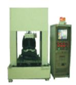
Equipment for inspecting disconnection, short circuit, overheating of the heater wire components mounted on a vehicle seat
