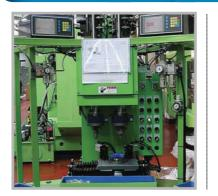
This equipment is the inspection / production equipment that automatically inspects the indentation load / indentation depth.
