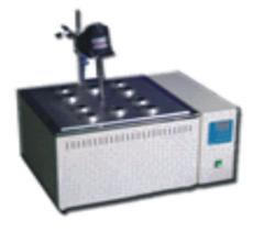
It is to test the quality and properties of various materials by heating a specimen while being stirred in oil and at a high-temperature; it consists of four test tubes, and four specimens can be measured at the same time.
