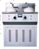
It is widely used to polish metal or implement consistent thickness.
