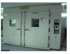
It is a test device combined with infrared heat resistance test and constant temperature and humidity test of various materials and products. It tests the heat resistance, light resistance and durability of products. The heat resistance test using an infrared lamp can be arbitrarily adjusted from 90°C to 120°C by controlling the infrared heat quantity.
