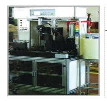
This equipment tests the LEAK of the AL housing part of the reducer and automatically applies the grease to the BEARING part of the second gear.
