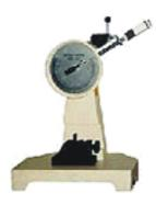
A device to measure the impact strength, a measure of tension
