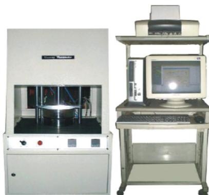
This test machine measures the Mooney viscosity, the lowest pattern viscosity and the scorch test of rubber based on the ASTM standard test method.
