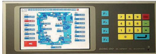
Display the shape of the product on the LCD screen and display the DATA on the measurement area. Product shape DISPLAY is OPTION.
