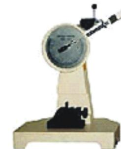
A device to measure the impact strength, a measure of tension
