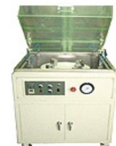
Equipment to check the surface condition of specimen by spraying water of 10 bar in four directions while moving specimen table up and down and constant rotating
