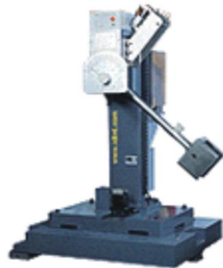
Test equipment to measure energy absorption
