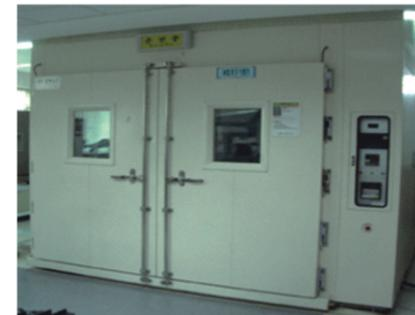
It is a test device combined with infrared heat resistance test and constant temperature and humidity test of various materials and products. It tests the heat resistance, light resistance and durability of products. The heat resistance test using an infrared lamp can be arbitrarily adjusted from 90°C to 120°C by controlling the infrared heat quantity.
