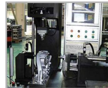
This equipment is used to simultaneously produce and inspect PIN with AL die casting products at a constant load / depth. The press-fitting of this equipment can work simultaneously on the Z-axis and X-axis, and it is possible to check the failure of indentation load accurately.
