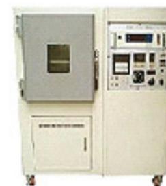
It has been designed / manufactured for the purpose of measuring heat deterioration of vulcanized rubber caused by ozone in the atmosphere and investigating / testing ozone resistance.
