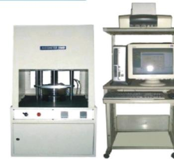
This tester shows continuous and stable curves in evaluating the properties of rubber, especially excellent in reproducibility of temperature.
