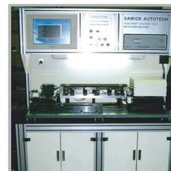
SHAFT DIA, RUN-OUT Inspection Equipment
