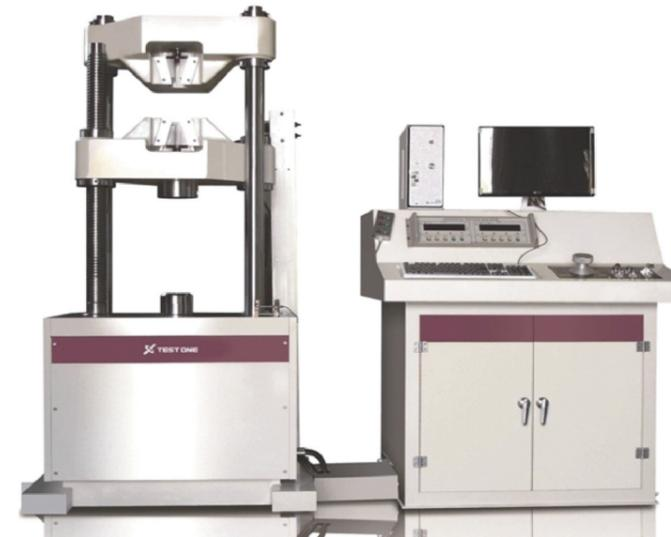
This is a hydraulic universal material tester beyond the conventional analog method and adopts a load detection sensor-high precision LOAD CELL or PRESSURE TRANSDUCER to digitally display the test load value and displacement; and it is also equipped with the computer to identify the test progress, analyze input and output data for efficient test and data management.
