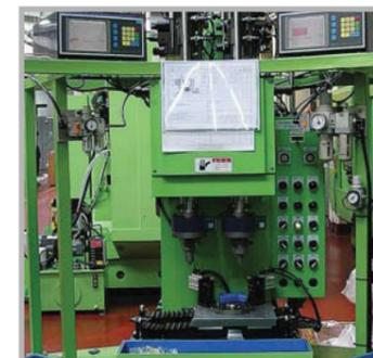
This equipment is the inspection / production equipment that automatically inspects the indentation load / indentation depth. The product is a system to press BEARING, PIN, and SLIP to the correct load and depth.
