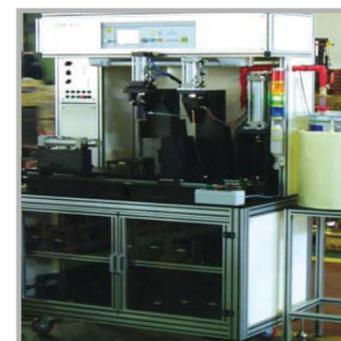
This equipment tests the LEAK of the AL housing part of the reducer and automatically applies the grease to the BEARING part of the second gear.
