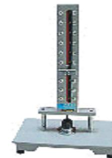
Used to evaluate the bond strength by applying impact to paint film and film.
