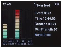
Live Cellular Mode showing two detected signals
