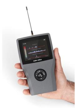
A simple, intuitive menu driven system displayed on a colour TFT screen allows the user to perform real time detection or to view events that have previously occurred. Each band has an individual 20 element signal strength meter enabling the precise source of a detected signal to be located with ease. An audible 'Beep' mode allows the user to monitor without looking at the display and a silent vibrate mode can also be used for particularly sensitive areas.
