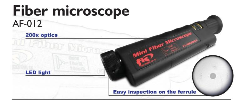
200x microscope designed for inspecting fiber ends, to look for dirt, impurities and oils that might interfere with signal transmission. It includes a universal 2.5 mm adapter for inspecting ST, SC or FC connectors, as well as a 1.25 mm adapter to inspect LC ferrule connectors. This microscope uses an oblique and coaxial LED light (powered by 2 AA batteries, included). Padded included.
