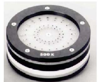
Surface Resistance Calibration Test Fixture
