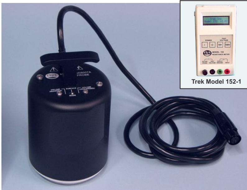
The Trek Model 152P-CR-1 Concentric Ring Probe is capable of measuring surface and volume resistance in materials as per IEC or ESDA standards. A three (3) position switch on the probe selects surface resistance or volume resistance measurements with either a guarded or unguarded outer electrode. (See page 2.)
