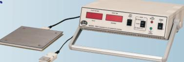
The Model 156A tests the efficiency of an ionizer's ion production by timing how long it takes air ions produced to discharge a floating plate that has been pre-charged to either a positive or negative value. The Model 156A also tests the balance between positive and negative air ions by measuring the offset voltage generated on a floating plate due to an imbalance of positive and negative air ions impinging on the plate from the ionizer.
