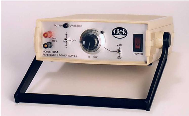
The Trek Model 605A is a high-voltage reference supply designed to provide precise control of output voltages in the range of 0 to +1 kV DC or 0 to -1 kV DC with an output current range of 0 to  $\pm 1$  mA DC.
