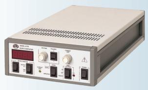
The Model 677B is a high-voltage power amplifier/supply designed to provide precise control of output voltages. It can be operated in one of two modes: as a high-voltage amplifier when it is configured as a noninverting amplifier with a fixed gain or as high-voltage power supply that responds to front panel controls to command exact output voltage or current.
