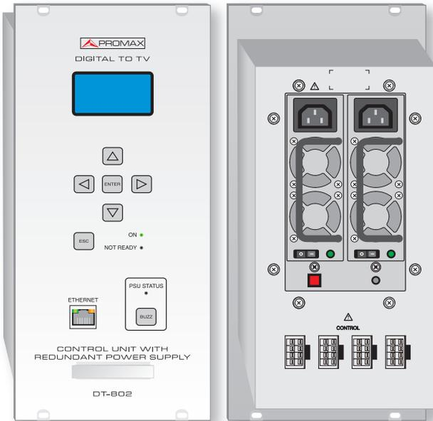
The **DT-802** is the control module of the "Digital To TV" system, with a dual redundant power supply of 300 W and two inputs for 1 or 2 different electricity suppliers. Each power module is individually removable and hot-swappable.
