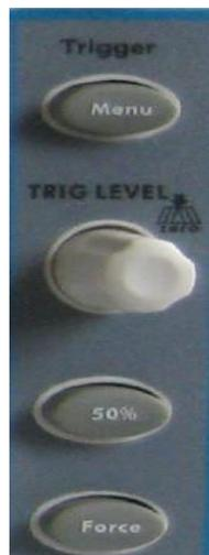
**Figure 14.** Trigger Control Zone.
