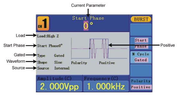
Figure 27: The User Interface of Gated Burst
