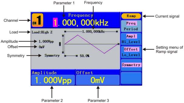
Figure 9. The User Interface of Ramp signal.
