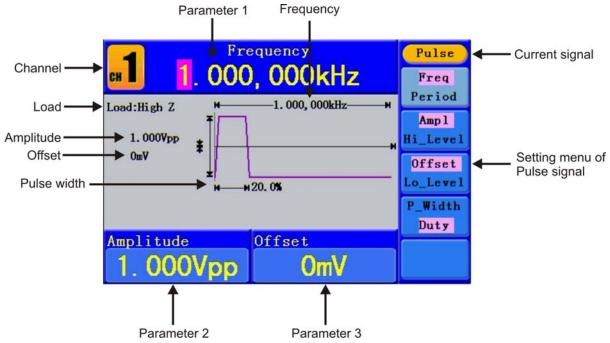
Figure 11. The User Interface of Pulse Signal.
