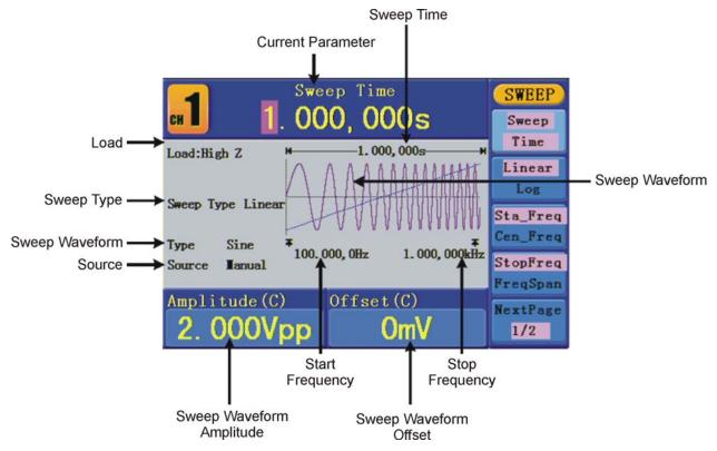
Figure 25: The User Interface of Sweep Mode
