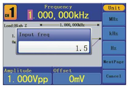
Figure 6. Set the frequency using number keys.
