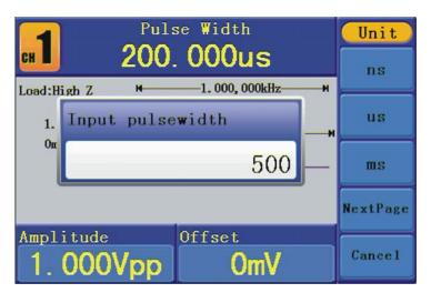
Figure 12. Set the Pulse Width of Pulse signal.
