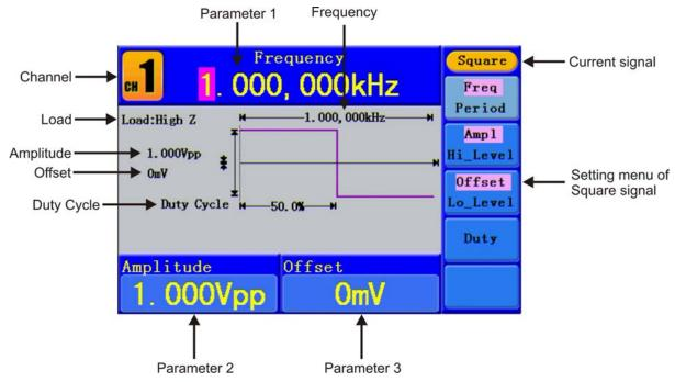
Figure 7. The User Interface of Square Signal.
