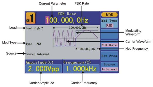
Figure 24: The User Interface of FSK
