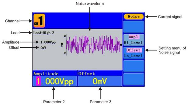
Figure 13. The User Interface of Noise Signal.
