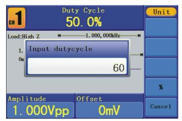
Figure 8. Set the Duty cycle of Square signal.
