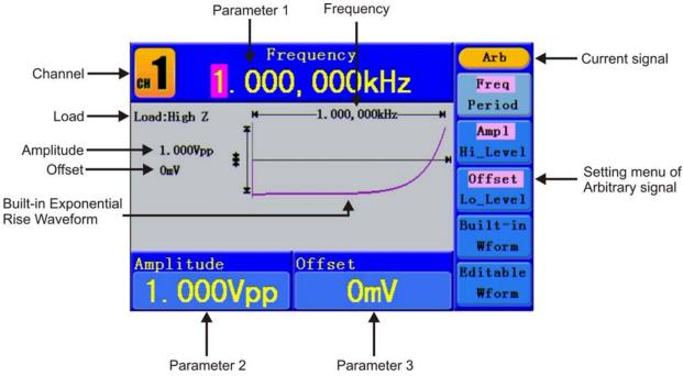
Figure 14. The User Interface of Arbitrary Signal.
