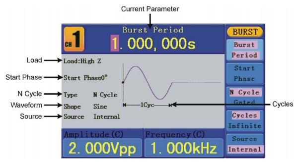
Figure 26: The User Interface of N-Cycle Burst
