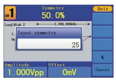
Figure 10. Set the symmetry of Ramp signal
