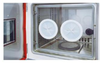
• Minimized temperature and humidity changes and observation of internal samples enabled.
