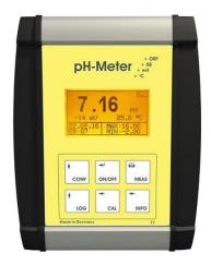
**Measurement value:** pH -2.00...16.00; -2000...2000 mV; Temperature: -10.0...100.0 °C; ISE
