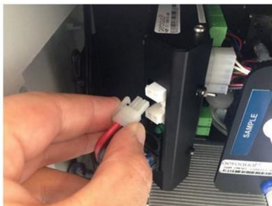
Figure 6-15 Fit the vacuum gauge, adjust the valves. Then stop the pump by removing power from the module, observe the change in pressure. If the leak rate is greater than 10 kPa in 10 seconds, then there may be a leak in the system. Check all the tube connections.
