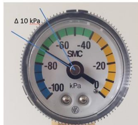
Figure 6-15 Fit the vacuum gauge, adjust the valves. Then stop the pump by removing power from the module, observe the change in pressure. If the leak rate is greater than 10 kPa in 10 seconds, then there may be a leak in the system. Check all the tube connections.
