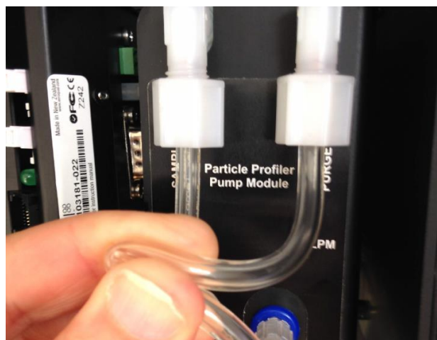
Figure 6-17 Pinch the tube with the newer Particle Profiler pump module
