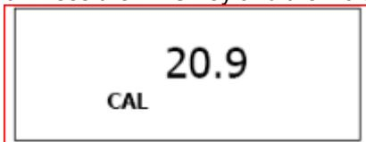
7. Press the Enter key. The device counts from 30 to 0, then returns to normal measuring operation and finishes the calibration. The calibration process takes 30 seconds.
