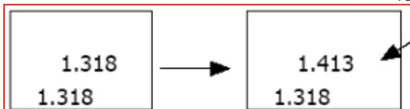
10. Press the Enter key so that the data are saved and the calibration is finished.
