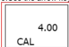
for calibration by means of a solution with a pH value of 4
