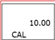
for calibration by means of a solution with a pH value of 10
