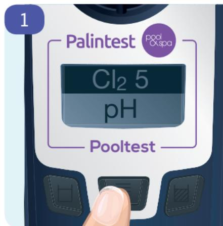
Select a test by pressing the Menu key. Scroll through the list until the desired test is highlighted.
