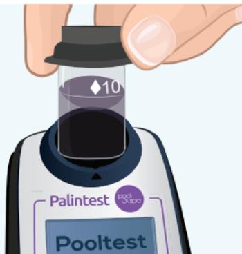
Prepare a 10mL sample by adding reagents according to the Test Instructions. Place this sample tube in the cell holder.
