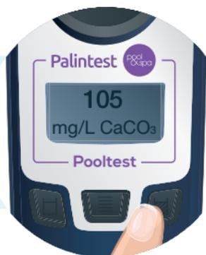
**Calcium Hardness - Calc & Calc NaCl****Colour Change:** Violet to Orange**Range:** 0 – 500 mg/L CaCO<sub>3</sub>**1**
