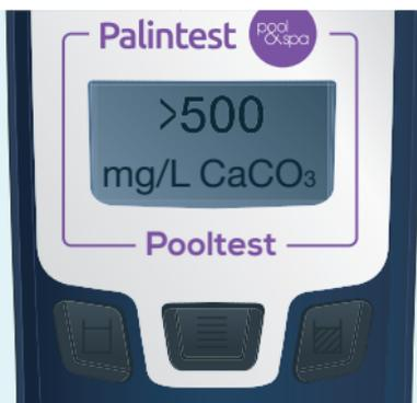
If a result is above the range of the test a '>' symbol will appear in front of the result. In this case it will be necessary to dilute the sample with deionised water and repeat the test.
