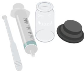
Rinse all equipment thoroughly with the water that is being tested.
