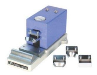
This tester is used to conduct an exfoliation test on the tiptoe of shoes. The operator is to press the exfoliation nail to the tiptoe and read the scale when the tester is exfoliating the test specimen.
