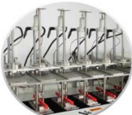
Specimen and weight holder can rise and descend automatically.
