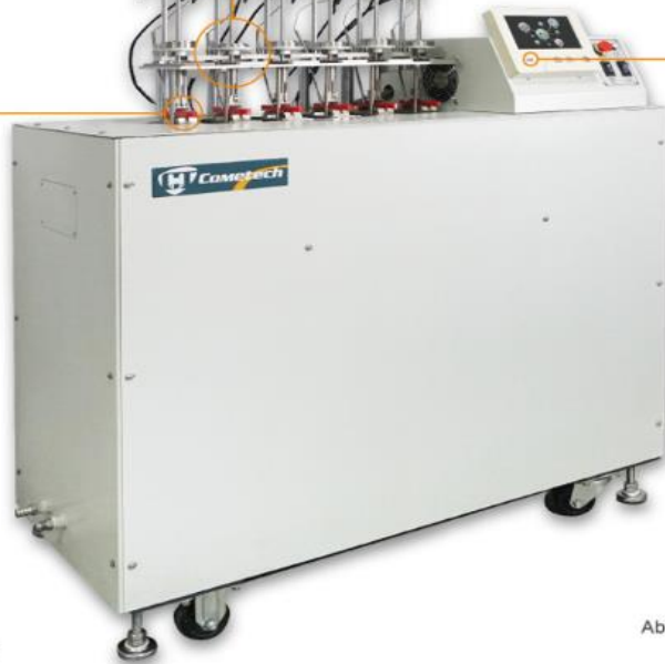
Equipped with high accuracy LVDT to measure the displacement.
