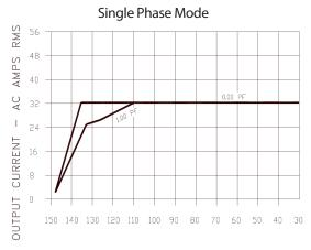
Short term overload s to 40A are permitted. Operating time before thermal shutdown or circuit breaker trip varies from seconds to severa; minutes depending upon line and tempertature conditions.
