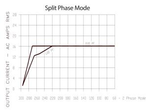
Short term overload s to 20A are permitted. Operating time before thermal shutdown or circuit breaker trip varies from seconds to severa; minutes depending upon line and tempertature conditions.
