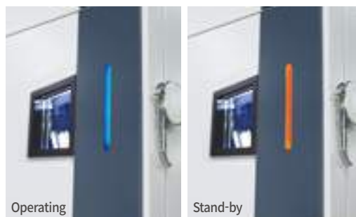
Indicator LED of operation condition.
