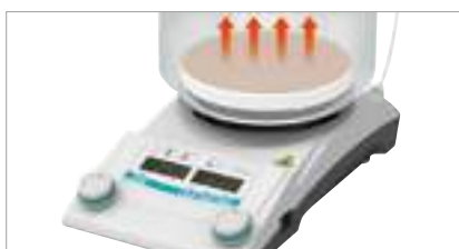
Top plate with excellent heat transfer.
