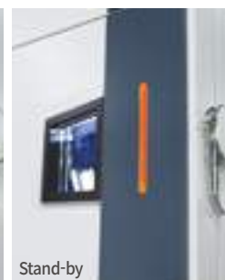
Indicator LED of operation condition
