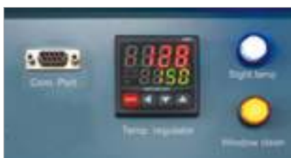
Electronic over temperature shutdown system.
