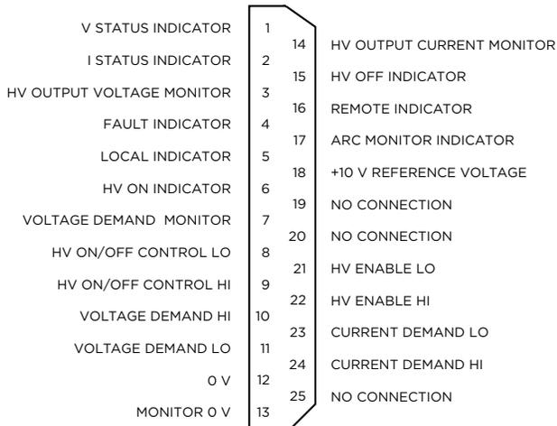
All logical indicators are open collector outputs rated at 16 V (max) in the off state. An internal 100 Ω resistor is connected in series with the open collector transistor. The pull down voltage is 0.9 V plus the internal resistor drop.
